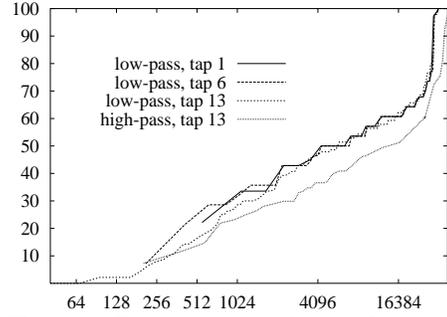
Figure 3. Fault coverage for on-line test
