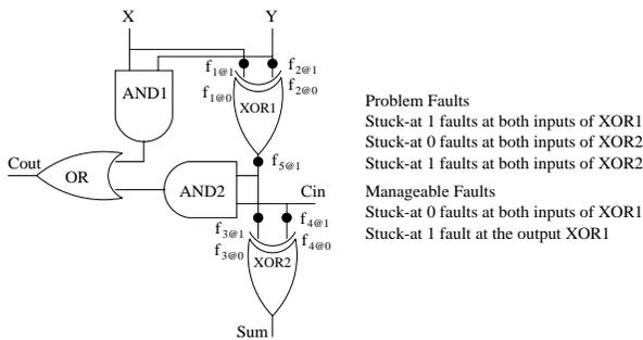
**Figure 4. A typical full-adder implementation**
