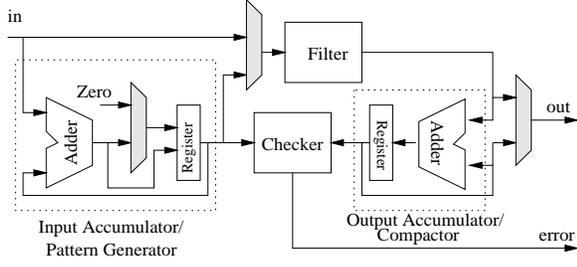
Figure 1. On-line/off-line BIST hardware
